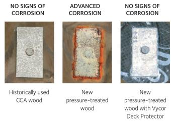
GALVANIZED METAL AFTER 1 MONTH, CONTINUOUS WET CONDITIONS. (NOTE: Red rust indicates ADVANCED CORROSION of galvanized coating)
